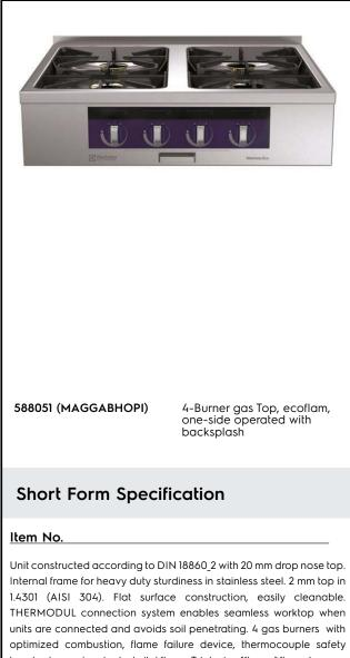
hand valve and protected pilot flame. Triple ring "flower" flame burners with anti-clogging design. Manual gas valves allow precise flame intensity control. Large pan support in cast iron with long center fins for various pan sizes. ECOFLAM pan detection system to save energy and to reduce unnecessary heat radiation in the kitchen. Deep flat spillage tray with rounded corners and drain hole. Metal knobs with embedded hygienic silicon "soft" grip enable easier handling and cleaning.
